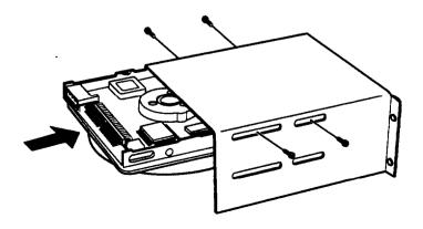
6. Place the bracket into the computer as shown below and secure it to the back panel with the four screws you removed from the back of the computer.
